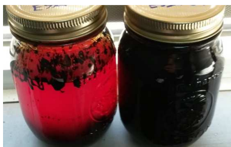
Figure 2: Wood vinegar (left) and bio-crude oil (right)
